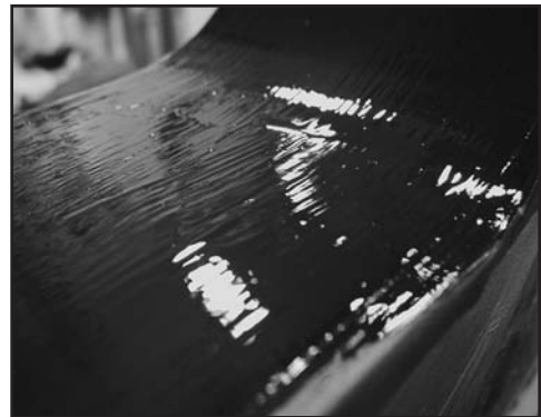
An oil-based pore filler on rosewood sides.
