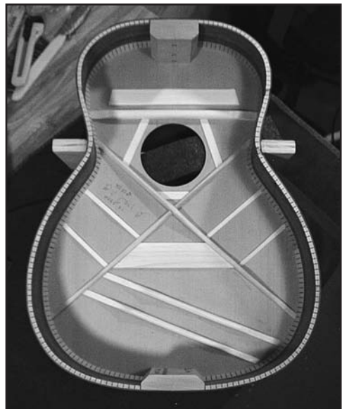
Internal mold removed ... back goes on next.
