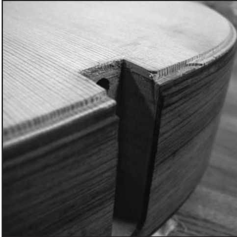
The opening is cleared for the neck tenon. Note the too-deep channel for purfling: One step toward learning the rule: "Test On Scrap!"
