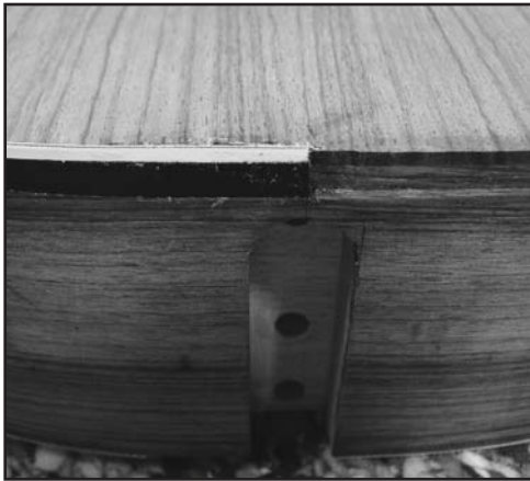
First mistake (routed channel too deep) and the "fix." Best I could do. Mistakes are part of the process; reading and thinking will prevent some, but not all.
