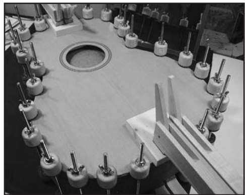
One way of clamping the top for gluing. Other ways are faster.
